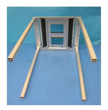
With the top (or bottom) on it's side, attach and tighten the four corner posts using the square washers with the notch facing out. Make sure the plastic gear is facing in as illustrated
