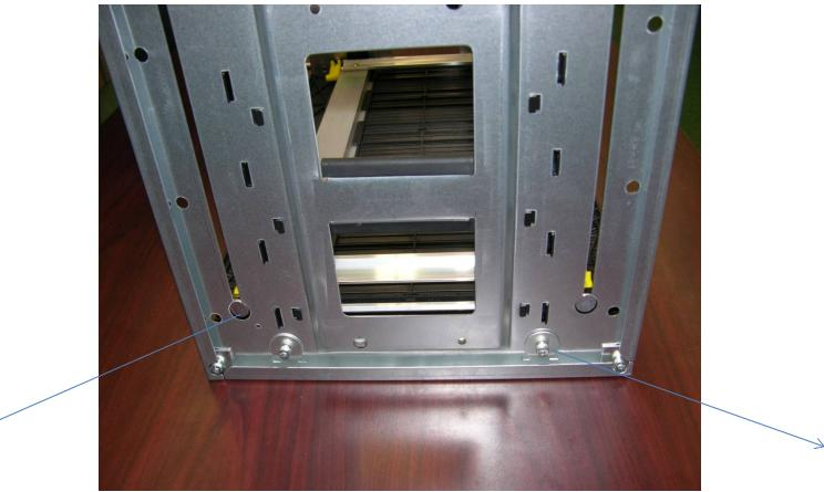
This shows the round end of the adjustable card guide aligned with the round hole and also shows the where the fixed card guide is attached with the round washers and SHCS
