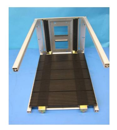
Lay the fixed card guide, slots facing up, on the two corner posts and attach one end using the SHC screws and round washers. It should be obvious where this card guide is attached as the adjustable card guide will be inserted into the keyhole so it can move in the slot
