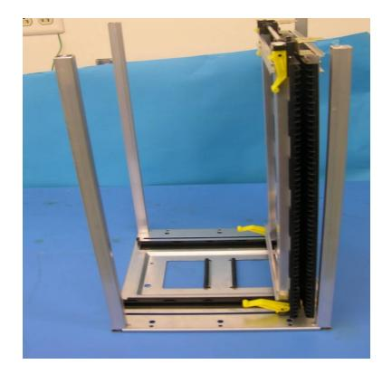
Stand the rack up and insert the adjustable card guide by inserting the round ends into the round holes on the bottom plate. Use the SHC screws and round washers to attach and tighten
