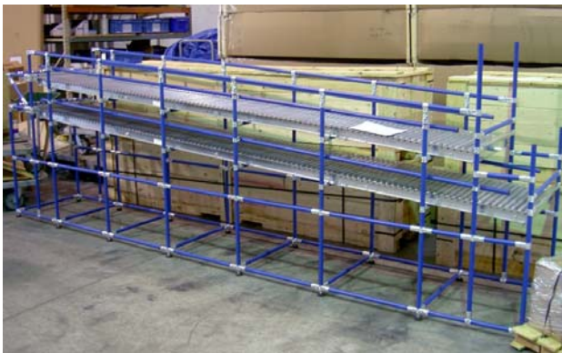
FLOW RACK W/ STEEL ROLLERS AND METER
