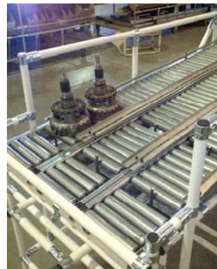
FLOW RACK W/ STEEL ROLLERS AND METER
