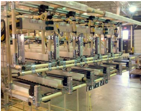
FLOW RACK W/ PICK-TO-LIGHT SYSTEM
