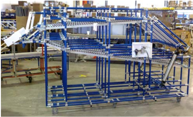
FLOW RACK W/ PNEUMATIC LIFT ASSIST FOR LOAD END
