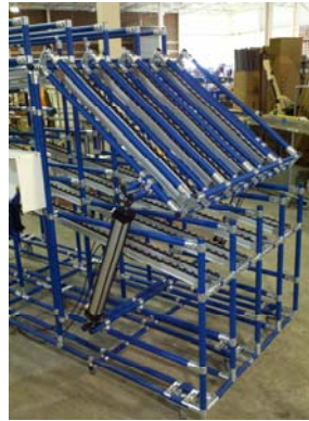
PNEUMATIC LIFT ASSIST FOR LOAD END
