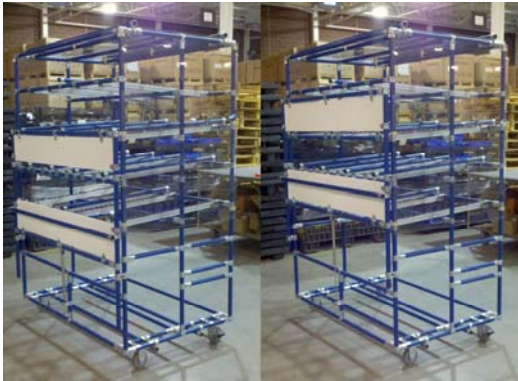
FLOW RACK W/ GAS SHOCK ASSISTED ACCESS DOOR
