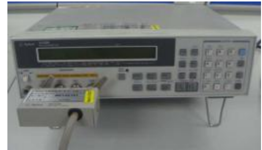
Milliohm Meter (Agilent): LLCR Test
