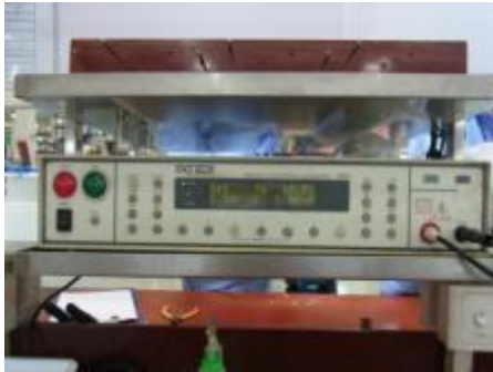
Hi-pot Tester (Extech): Insulation Resistance & Voltage Proof Test
