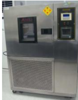
Humidity Chamber (Asli): Thermal Cycling Test
