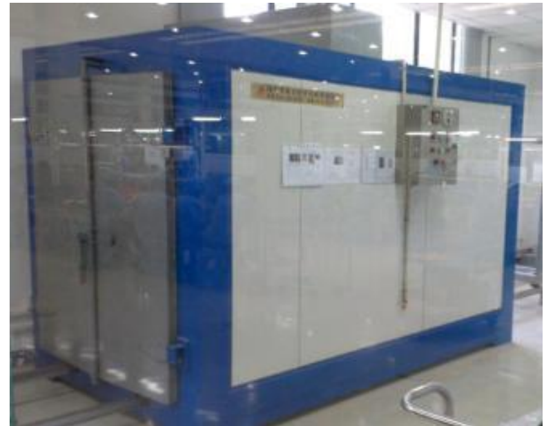
Oven (Powder is solidified in high temperature)
