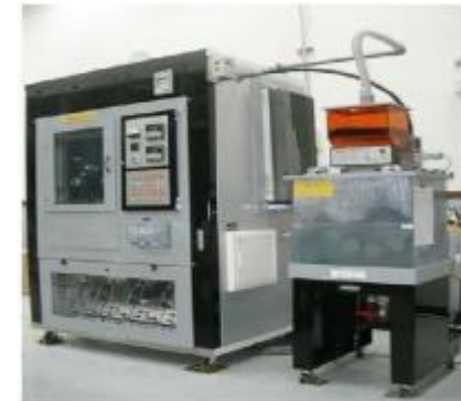
MFG Chamber (Yamasaki): Mixed Flowing Gas Corrosion Test
