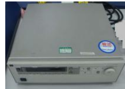
Power Supply (Agilent): Current Rating (T-rise) & Contact Resistance Test
