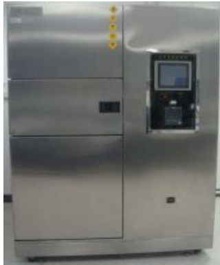
Thermal Shock Chamber (Asli): Thermal Shock Test
