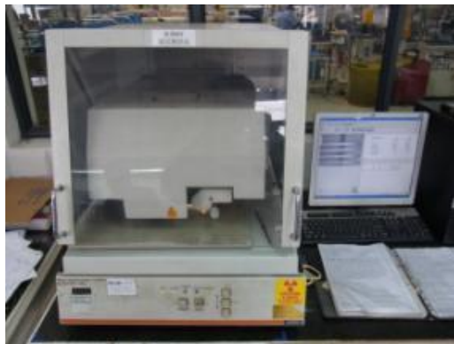
X-ray (Fischer): Plating Thickness Measuring
