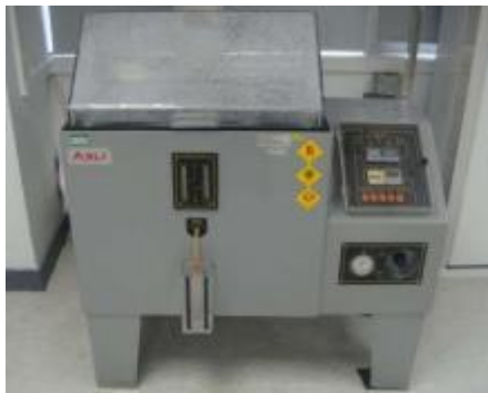
Salt Spray Chamber (Asli): Saly Spray Test
