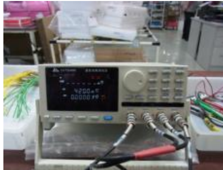
Micro-ohm Meter (Hope tech): Resistance Test
