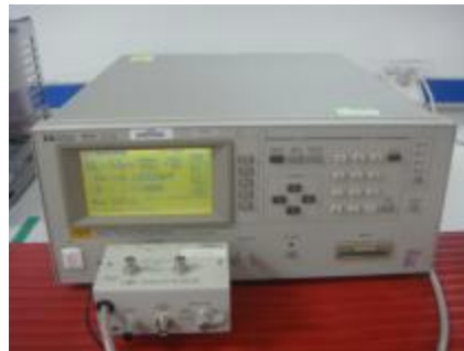
Precision LCR Meter (HP): Capacitance Measuring
