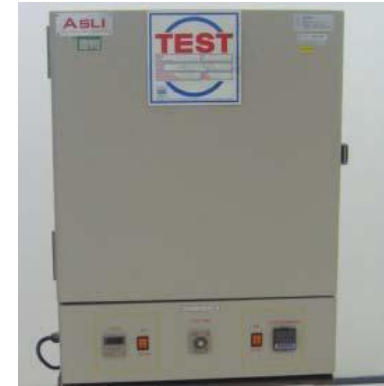
Oven (Asli): High Temperature Life Test
