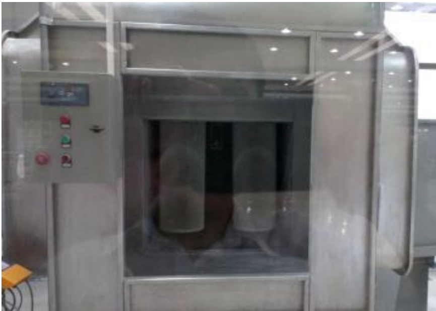
Spray chamber (Powder is absorbed on the surface of conductor under electrostatic effect)
