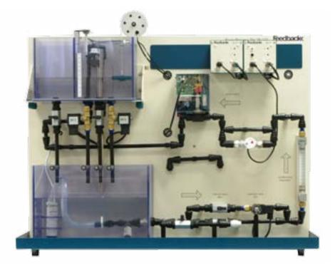
The Level/Flow Process Trainer is a single loop system allowing the study of the principles of process control, using liquid level and flow rates as the measured process variables. The system is a completely self-contained, low pressure flowing water circuit supported on a benchtop-mounted panel, making it suitable for individual student work or for group demonstrations.
