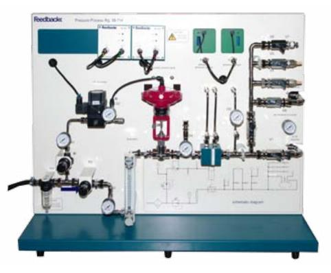
The Pressure Training System is a single loop pneumatic control system. It enables the study of the principles of both pressure regulation of a process and the control of flow in a pressurised system.
