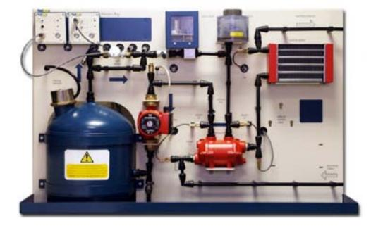
The Temperature Training System uses water as the process fluid which allows the study of the principles of process control using primary and secondary circuit temperatures as the process variables to be controlled.
