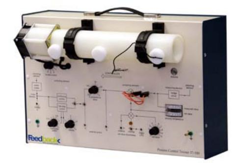
The 37-100 Process Control Trainer teaches the basic ideas of process control to technicians, process operators and control engineers.
