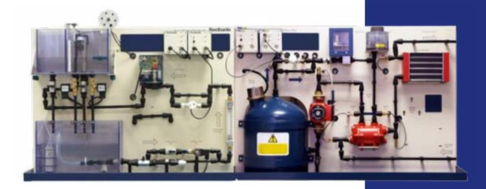
The combined Level/Flow and Temperature Process Control System is self-contained and has all of the features of the individual Level/Flow and temperature systems plus Remote Set Point Control.
