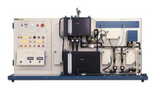
The Industrial Process Trainer has been designed to teach a methodical approach to fault diagnosis in industrial processes. The methodologies taught within the system are equally relevant to any student or trainee studying fault diagnosis. Faults can be introduced by the instructor via switches concealed behind a locked compartment, to which the student does not have access.
