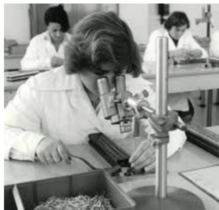
HANDMONTAGE VON FEDERKONTAKTSTIFTEN, 1980 HAND ASSEMBLY OF SPRING CONTACT PROBES, 1980
