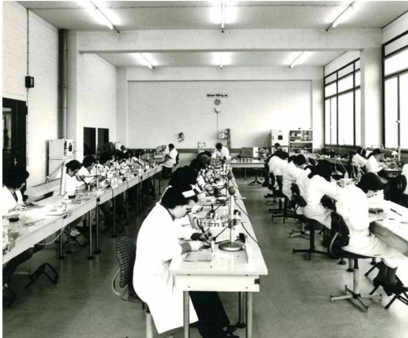
DER FEDERSAAL: HAARDÜNNE METALLBÄNDER WERDEN ZU FEDERN GEFORMT SPRING HALL: METAL BANDS AS THIN AS HAIR ARE FORMED INTO SPRINGS
