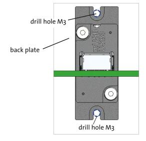
Make a sufficient cut to push the test conenctor through to the back. Plan at least 1 mm of space between notch and test connector.
