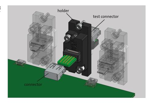
Align the median level of the connector to be tested and of the test connector.
