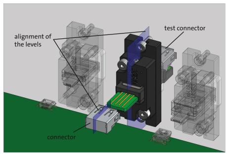
Align the lower level of the test connector to the lower internal level of the connector to be tested.
