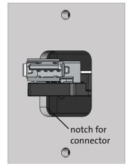
For mounting the test connector loosen the retaining screw. Insert the test connector into the connector to be tested on stop at the bottom. Move it back about 0.5 to 1 mm in order not to risk a damage of the connector to be tested. Tighten the retaining screw of the connector.
