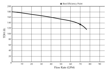
The curve reflects maximum performance characteristics without exceeding full load (Nameplate) horsepower. Operation is recommended near the Best Efficiency Point. Operating at the outer limits of the curve is not recommended. Performance curves are based on actual tests with clear water at 70° F. and 1280 feet site elevation.
