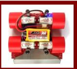
Using the standoffs, four screws, and the large 5/64" hex wrench, attach the scoop to the top of the chassis and the metal ballast plate to the bottom with the four washers spacing it from the pcb. Don't forget them or short circuits will damage the board and battery!
