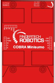
The Cobra has two on-board motor drivers (left and right). To operate them, you will need to connect their DIR (direction) and PWM (speed) pins to a microcontroller. For DIR, 5V is forward direction and 0V is reverse. The PWM pins require a 5V pulse-width-modulated waveform for smooth operation.
