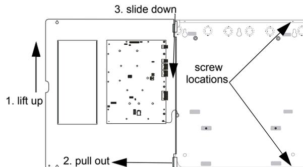
**Figure 1 Removing the Dress Panel**
