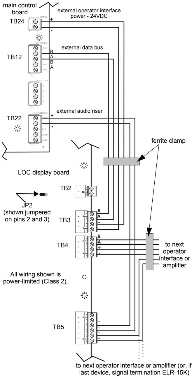
**Figure 4 Local Operator Console Wiring (Class B/Style Y)**
