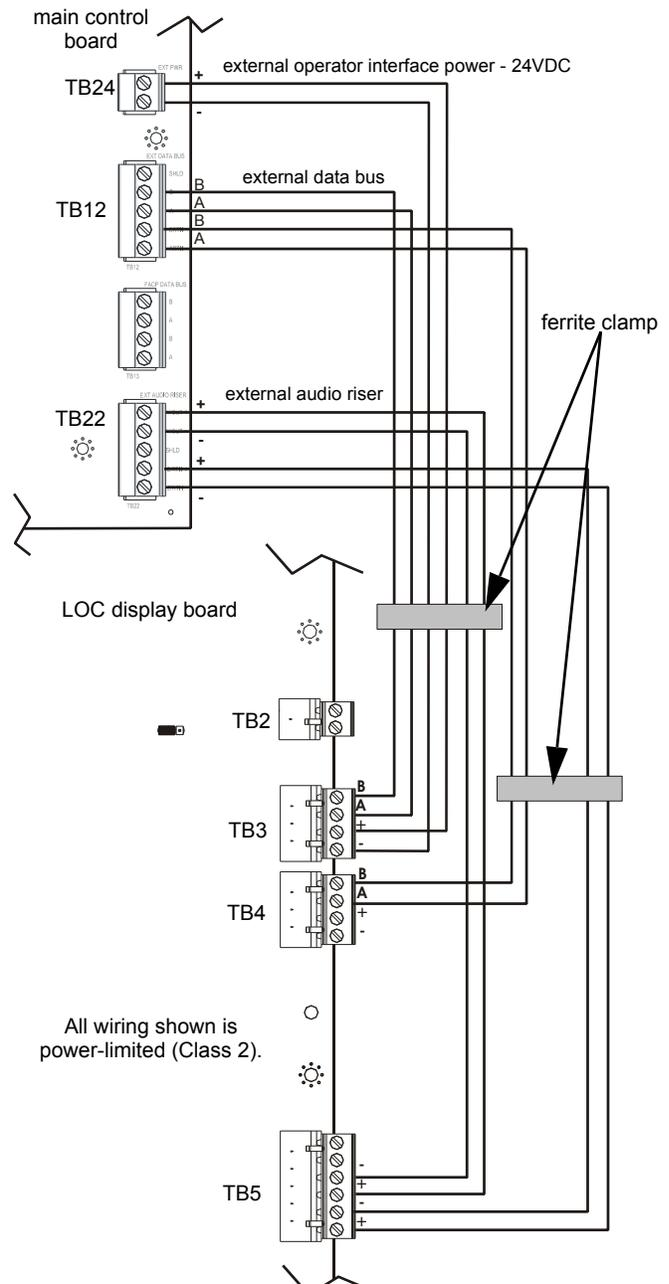
**Figure 5 Local Operator Console Wiring (Class A/Style Z)**
