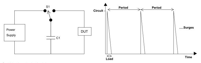
S1: High-voltage insulated switchC1: High-voltage variable capacitorPower supply: Variable 0 ~ 50KV DC
