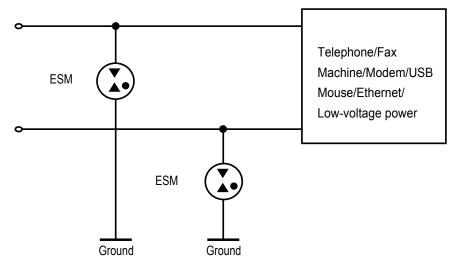
These ESM absorbers protect against common-mode interference voltages, i.e. surge voltages that appear in both exchange lines connecting to the ground. in the event of voltage overload, the ESM protects both exchange lines by conducting the surge current away to the ground.
