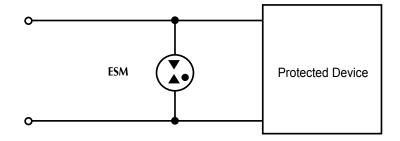
Signal circuits often run with no ground conductor. A ESM circuit located between the two signal lines offers differential mode protection by preventing the occurrence of large potential difference at the input of the equipment to be protected
