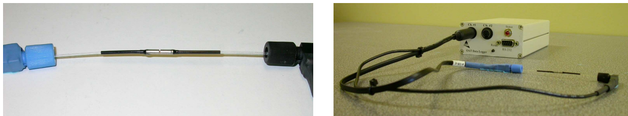
Figure 1 : Left: OAT-TS sensor connected to RGB light source and to light detector. Right: OAT-TS sensor connected to OAT-DL signal conditioner (2 channels).
