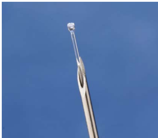
Figure 1 : Fiber Optic Sensor FOP-MIV ( \varnothing 550 \mu\text{m} ) pictured here in a 24 gauge needle.
