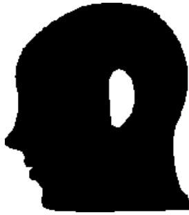
Fig. 1. A proposed 6 mm thick smooth lossy ear phantom to obtain peak 1- and 10-g SARs within \pm 10-15\% of those obtained for anatomically-realistic models. This model with the lossy ear replaced by a 6 mm thick plastic ear ( \epsilon_r = 2.56 ) gives SARs that are a factor of 2 or more lower as given in Tables 1, 2.
