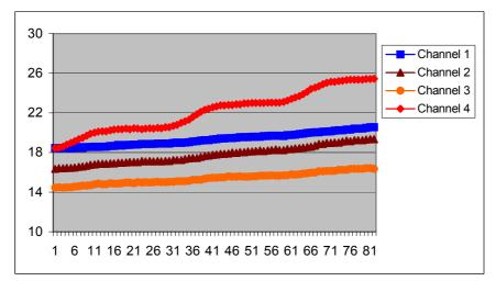
Figure 2 Temperature – time profile of chicken breast at 2450 MHz (200 Watts, 60 sec) without turn-table on.
