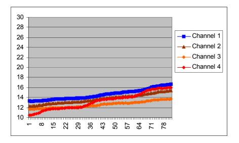
Figure 1 Temperature – time profile of chicken breast at 2450 MHz (200 Watts, 60 sec) with turn-table on.
