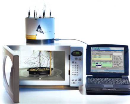
Figure 9: Commercial kitchen MW oven instrumented by FISO Technologies for multiple point-sensing with F-P temperature sensors.
