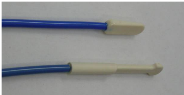
Figure 10: Example of medical OFS assembly developed by FISO Technologies for skin surface temperature sensing of patient during MRI procedure. The diameter of the blue cables is 3 mm.
