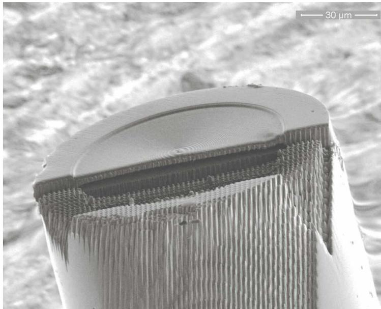
Fig. 7. SEM photo ( $\times 2000$ ) of the diaphragm cross-section showing the entrapped air cavity and the suspended recessed diaphragm. The sensor was cut by scanning ion-beam creating the apparent roughness visible in the front of the sensor fiber
