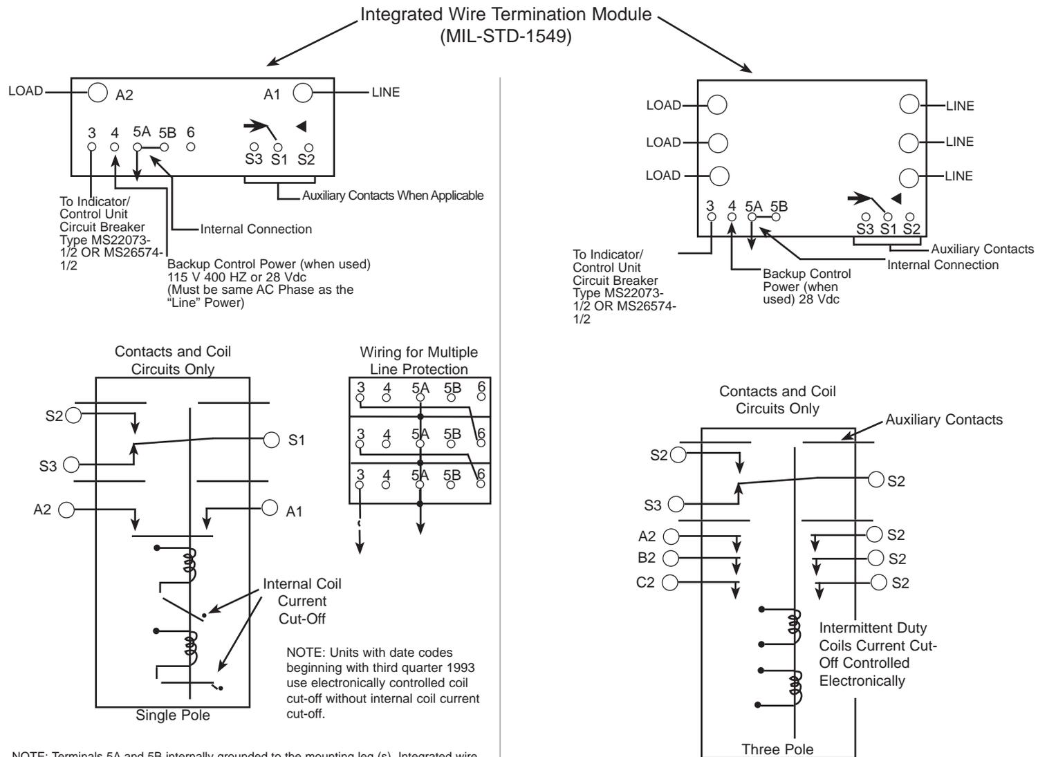
NOTE: Terminals 5A and 5B internally grounded to the mounting leg (s). Integrated wire termination (IWT) module accepts pin contacts P/N M39029/1-100 or -101. Use with insertion/extraction tool M81969/14-02.
