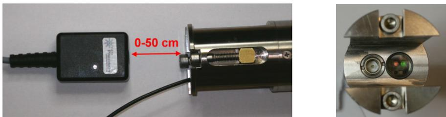
Picture: IR converter and logger top (without connected antenna)
