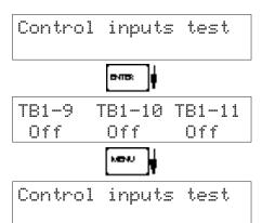
Press Enter to test the control inputs.
