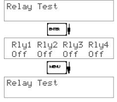
Press Enter to test the relays.
