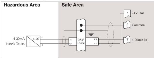
Return Temperature Input (4-20mA Transmitter)
