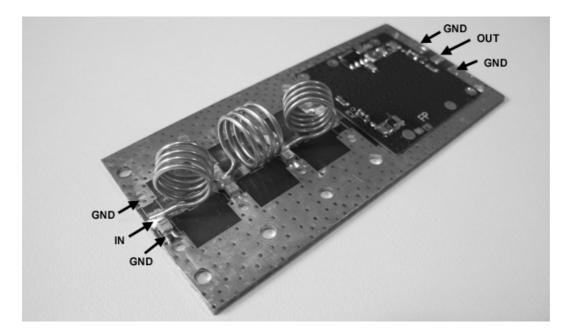
**IN**, connect inner conductor of 50 Ohm Teflon coax to this point. For best result use 18CM Coax length between your amplifier and LPF
