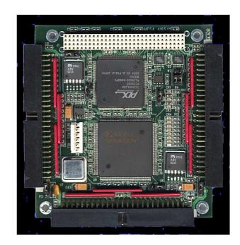
The MESA 4I65 is a general purpose programmable I/O card for the PC/104-PLUS bus. The 4I65 uses a 200K gate Xilinx FPGA for all logic, so it is truly an "Anything I/O" card.
