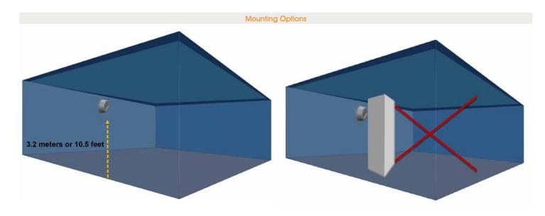
The long range sensor is best used as a wall mounted sensor. The recommended install for this sensor is 3.2 meters or 10.5 feet from the floor
