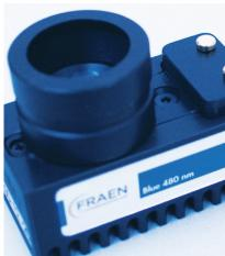
**FLUOLED® 1CFW and 3CFW** are designed for infinite focus optical microscopes providing a 23 mm field of view. A field diaphragm is available to size the illumination area.
