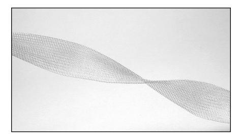
Ja-Bar manufactures a Monel mesh "tape" for electronic shielding applications. The mesh is used by simply wrapping the cable or harness assembly with the mesh, using a .250" overlap to insure proper continuity. The mesh wrap is then terminated one end, or preferably both ends, to the ground. The "tapes" are available in various widths as noted below. Physical make-up and Electrical characteristics are as follows:
