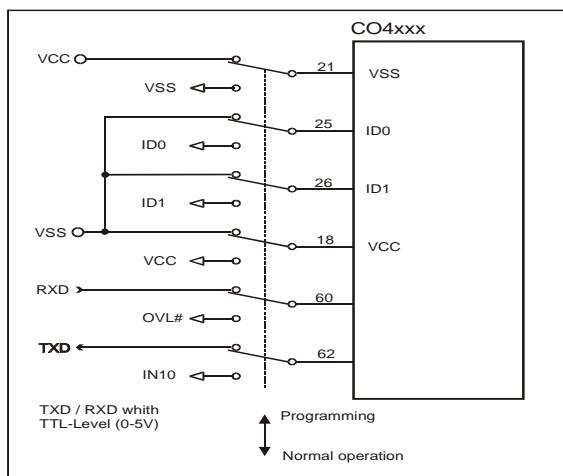
To enable the programming condition close the jumpers Jx and Jy.
