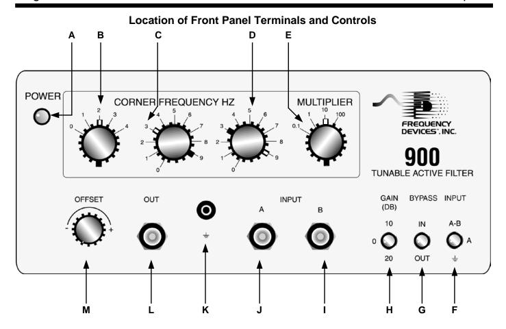
A. POWER Status Lamp: This red LED indicates whether or not the power to the analog filter circuitry of a Model 900CT/BT Series instrument is ON. With the power switch in the ON position, the LED glows continuously indicating internal DC power levels are correct. If LED does not light when power switch is in ON position, 1) reset instrument by cycling POWER switch OFF and ON, 2) Check line fuse.
