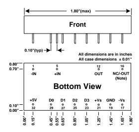
Note: NC pin is used as "-OUT" for differential input option.
