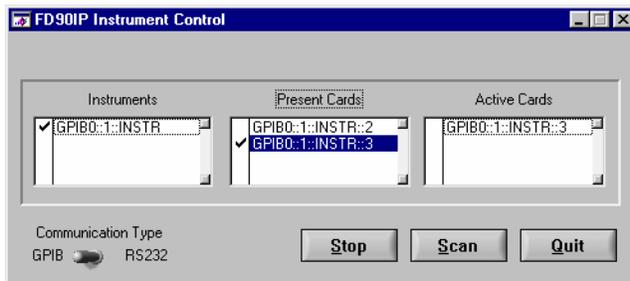
6. “**CLICK**” on **SCAN**, this will display an instrument list. “**CLICK**” or highlight the desired chassis, this will display an instrument list of slot cards installed in the 90IP chassis.
