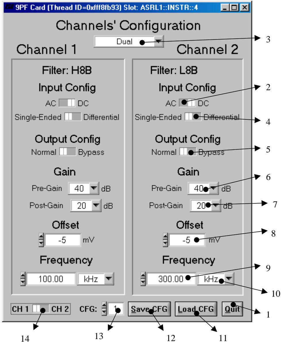
Figure 2 - Components of the Soft Front Panel.
