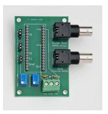
**Oscillators Available** D45 100 Hz to 50 kHz DX45 100 Hz to 50 kHz D45Q Quadrature 100 Hz to 100 kHz
