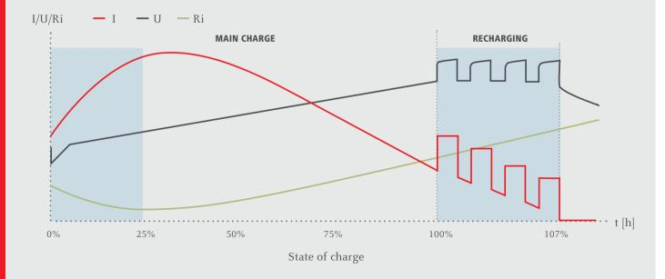
Adapting the current to the battery prevents charging losses when charging commences and during the recharging phase. The battery only receives the current that it actually needs.
