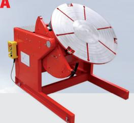
/ Rotilting positioner are universal applicable for manual and mechanized welding applications as well as for precise positioning of work pieces.
