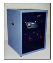
The PLS510 automatic tester is designed primarily to do SURGE testing either as single pulses or with Forward and Reverse bias, according to methods 4066-1 or 4066-2. In addition, it can also test VF with rectangular pulses and THERMAL RESPONSE either in DVF (mV) or degrees per watt. All three test types may be performed in a single test program.
