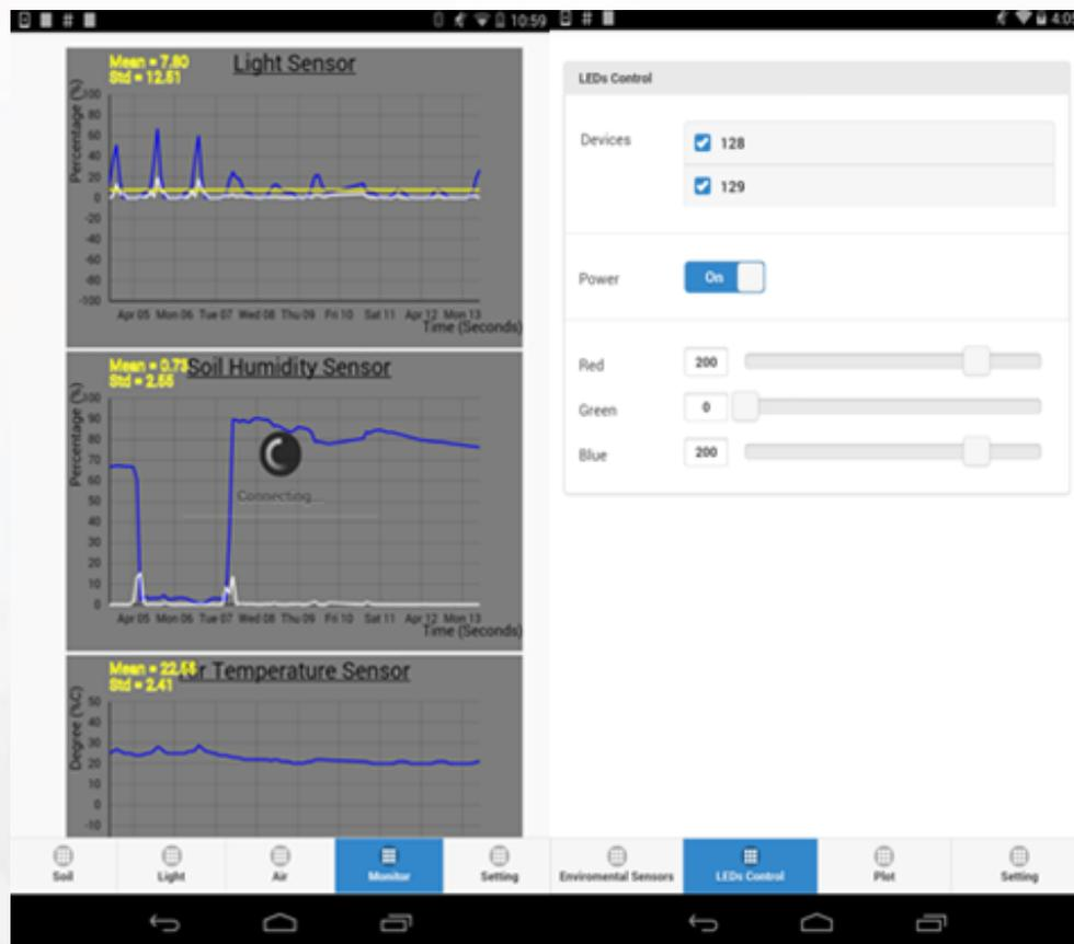
Figure 2: Android Application displaying data captured and transmitted from an FT900
