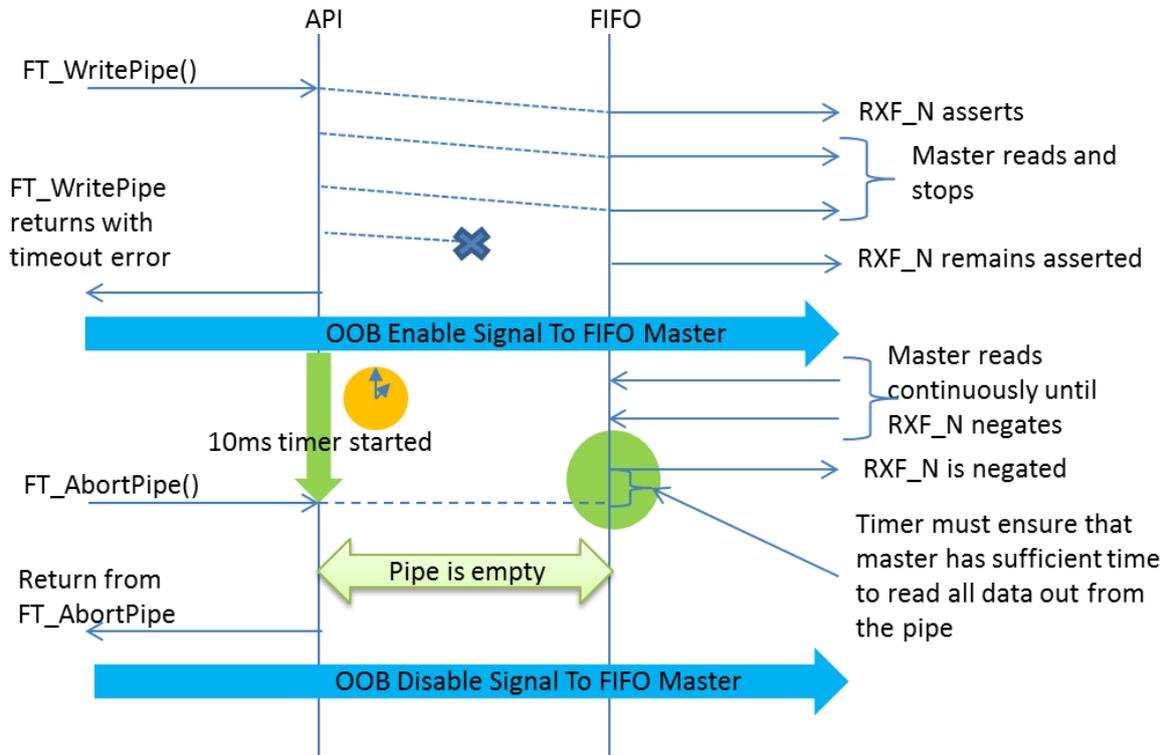
**Figure 5 - Write Pipe Abort Recovery**
