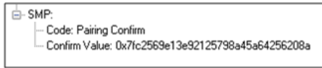
Figure 10 - Responder Pairing Confirm Example (ComProbe Frame Display, BPA 600 low energy capture)
