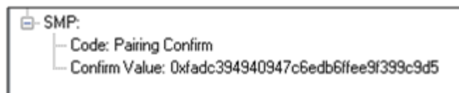
Figure 9 - Initiator Pairing Confirm Example (ComProbe Frame Display, BPA 600 low energy capture)
