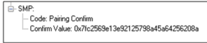
Figure 27 - Responder Pairing Confirm Example (ComProbe Frame Display, BPA 600 low energy capture)
