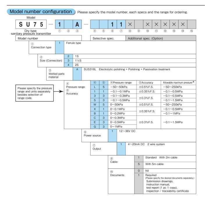
\* Please use it within the range of proofpressure of connected parts (clamp, nut, and gasket, etc.).
