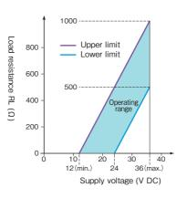
If you need more than 500  $\Omega$  load resistance, is required supply voltage over 24V DC.
