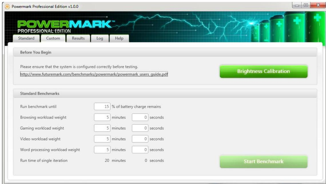
The custom tab lets you define your own test scenario by individually setting the per-iteration run times of each of the four workloads, as well as setting the battery charge end condition. See the specification included later in this document for details of each workload.
