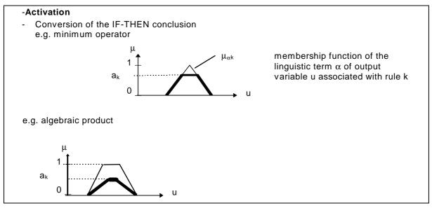
Figure A.2.3-2b: The principles of activation (by way of an example)
