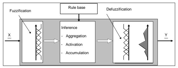
Figure A.2-1: Structure and functional elements of Fuzzy Control
