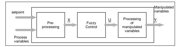
Figure A.3-2a: Fuzzy-based controller: Fundamental structure
