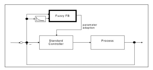
Figure B.2-1: Example of a parameter adaptation
