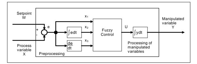
Figure A.3-2b: Example of a Fuzzy-based controller
