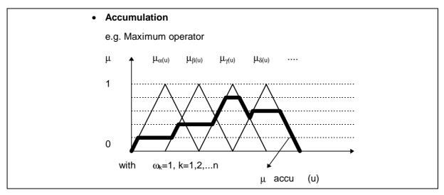
Figure A.2.3-2 c: The principles of accumulation (by way of an example)
