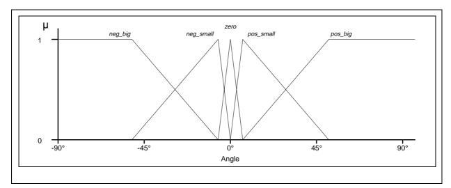
Figure C-3: Linguistic variable "Angle" of the container to the crane head
