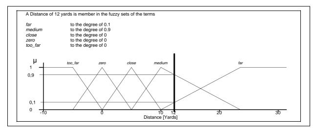
Figure C-5: Fuzzification of the linguistic variable distance
