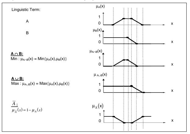
Figure A.1-4: Algorithms for implementing operations between two membership functions
