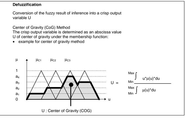
Figure A.2.4-1a: Methods of defuzzification
