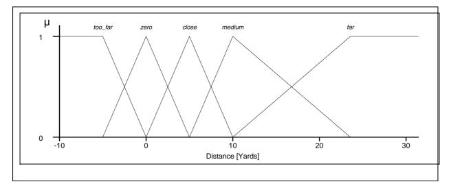
Figure C-2: Linguistic variable "Distance" between crane head and target position
