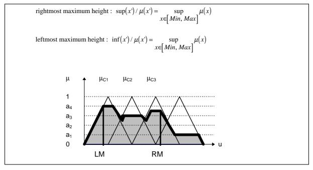
Figure A.2.4-1b: Difference between Left Most Maximum and Right Most Maximum
