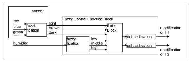
Figure D-2: Principle of the fuzzy based control of the oven
