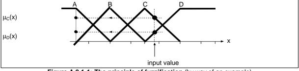
Figure A.2.1-1: The principle of fuzzification (by way of an example)
