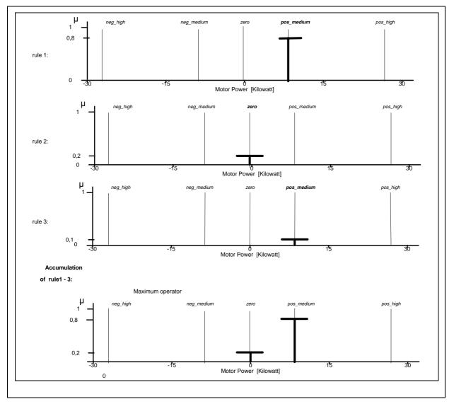
Figure C-13: Principles of Accumulation
