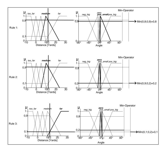
Figure C-9: Principles of aggregation
