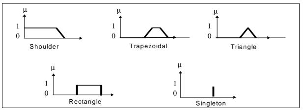
Figure A.1-3: Commonly used shapes of membership functions
