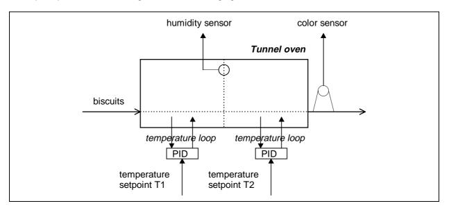
Figure D-1: Principle of the controlled system
