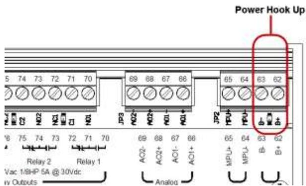
**NOTE:** Run power directly from battery posts to controller power terminals when battery is the power supply.
