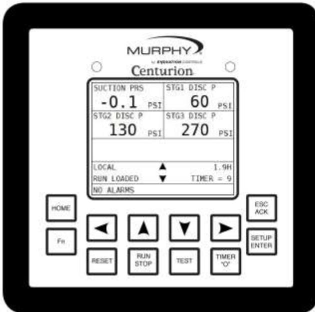
The display module is a highly integrated operator interface specially programmed to complement and support the Centurion controller. The primary purpose of the display is to:
