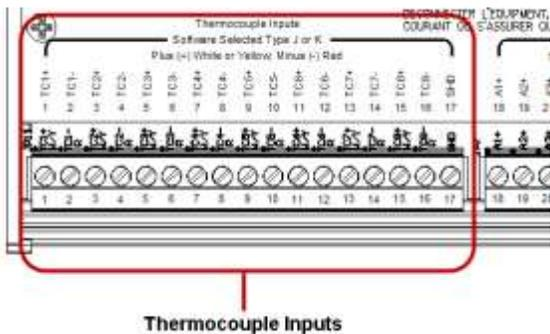
**NOTE:** An additional terminal connector is provided, identified as SHD, which isolates thermocouple shields. This connection, at terminal 17, is intended to be wired to an isolated bus bar for thermocouple shield wires. If shields are grounded, do not connect shields to SHD terminal. Connect all shields to SHD or to ground but never both.
