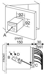
The AS710 is mounted in the front of a control panel through a DIN standard aperture,  $92 \text{ mm} (3^{5/8"})$  square.
