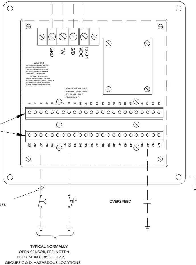
SENSOR SWITCH INPUT TERMINAL STRIPS
