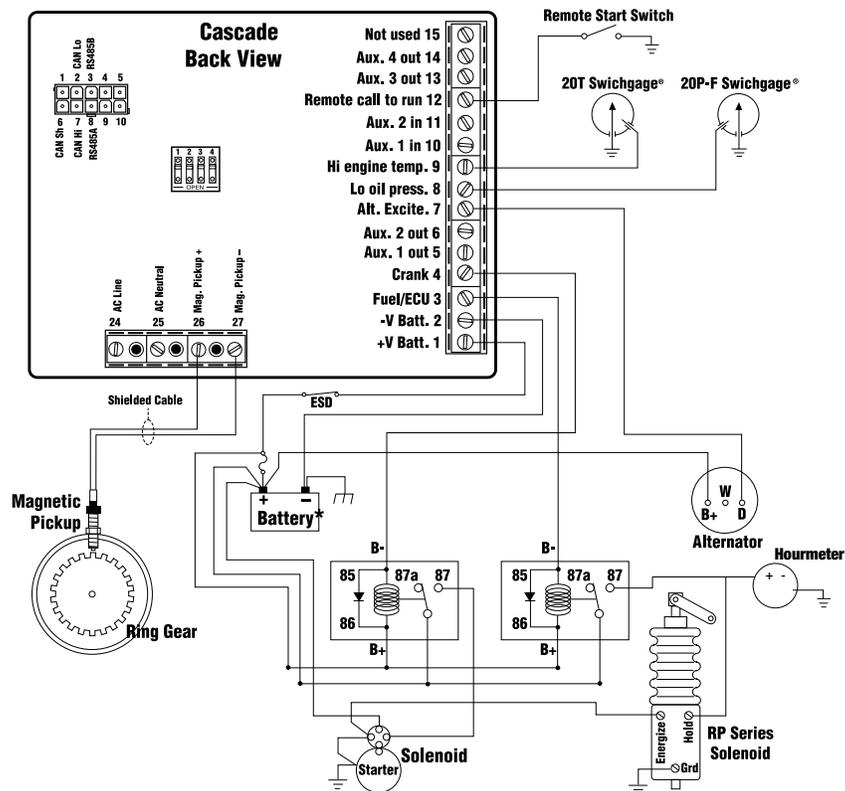
\*Always provide proper circuit protection with fuses or circuit breakers.
