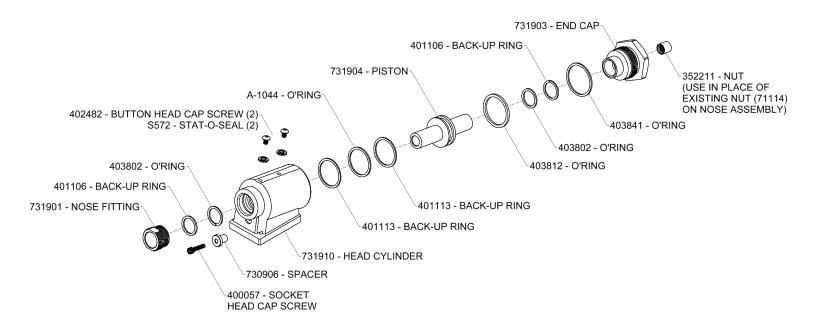
NOTE: Use nut (352211) in place of existing nut (71114) on nose assembly. Attach nut (352211) using tee wrench (A-291) supplied with tool.
