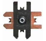
GAGE BILT ALSO SUPPLIES PIN & COLLAR SWAGE INSPECTION GAGES TO CERTIFY CORRECT SWAGE INSTALLATION.
