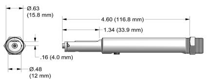
POINT NOSE ASSEMBY DOWN WHEN ATTACHING TO TOOL
