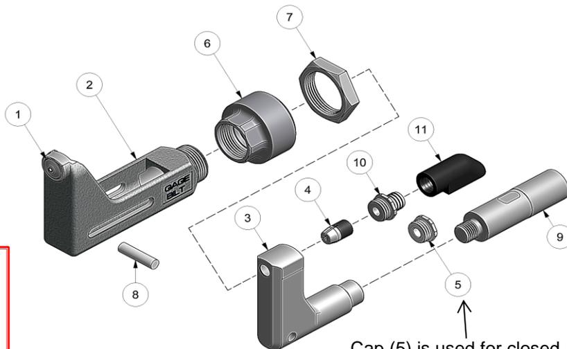
Cap (5) is used for closed access applications only or when clearance is an issue.
