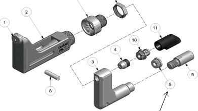
Cap (5) is used for closed access applications only or when clearance is an issue.
