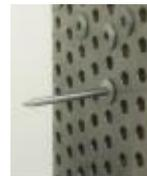
2. Insert fastener into nose assembly.
