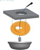
Insert the antenna into the hard ceiling adapter, push it towards the ceiling and lock it. ("a click sound should be heard") as shown in below illustration
