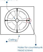
Center the hard ceiling adapter above the center hole and attach it with 4 countersunk head screws 1/8" (3.80mm) diameter suitable for the ceiling material (not provided).
